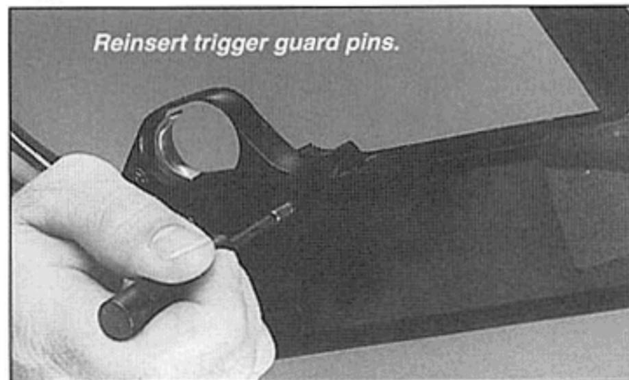
slide release lever engaged to the release button mechanism. You may need to press the slide release button to make the proper connection. Line up the holes in the trigger assembly with the holes on each side of the receiver.
