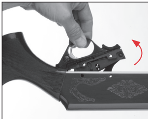
Lift the trigger group from the receiver.
