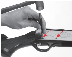
Tap the trigger group pins through the receiver.
