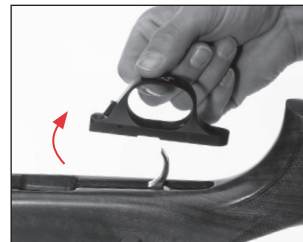
Carefully lift the trigger guard from the stock.
