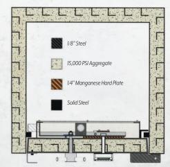
High-density aggregate concrete, steel fiber and improved adhesive resins combine to make the TL-30 significantly stronger than safes made with average, construction-grade concrete.
