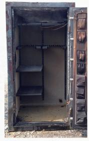
Browning ProSteel Safe with 1-7/8" thick insulation after 100 minutes at 1680° F.
