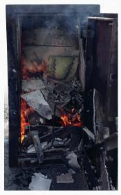
Leading U.S. built competitor safe with 1-7/8" thick insulation after 100 minutes at 1680° F.
