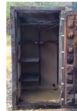
Browning ProSteel safe with 1-7/8" thick insulation after 100 minutes at 1680°.
