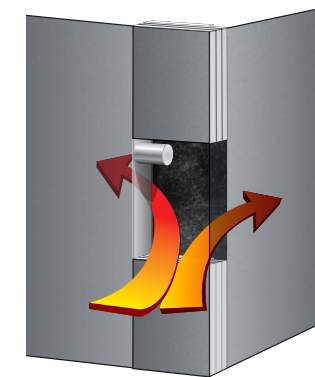
COMPETITORS' INTERNAL HINGE Internal hinges allow up to eight times more heat to radiate inside the safe through gaps in the fire insulation.
