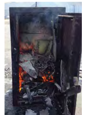
Leading competitor safe with 1-7/8" thick insulation after 90 minutes at 1680°.
