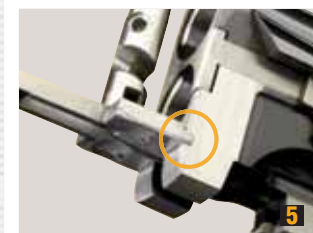
Tapered Locking Bolt
