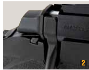
Bolt Lock Override Button
