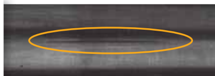
The competitor's choke tube is grooved and pitted after shooting 500 rounds of steel shot.
