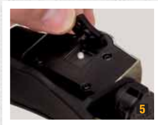
All-Weather Seals on USB Ports
