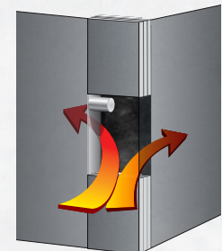
COMPETITORS' INTERNAL HINGE Internal hinges allow up to eight times more heat to radiate inside the safe through gaps in the fire insulation.
