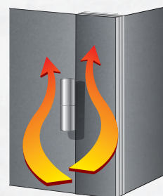
OUR EXTERNAL HINGES External hinges eliminate gaps in the fire insulation to block heat from entering the safe.
