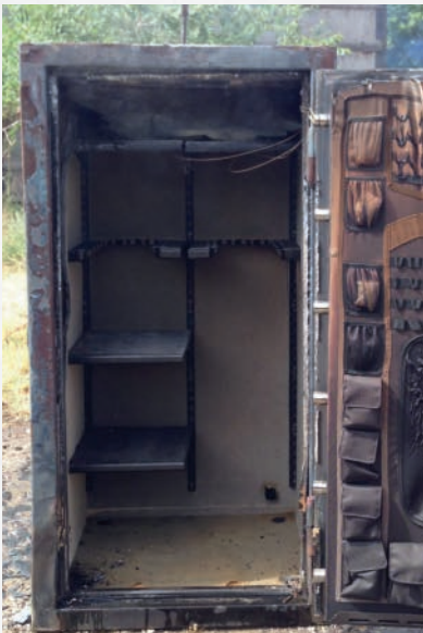
Browning ProSteel safe with 1-7/8" thick insulation after 100 minutes at 1680°.
