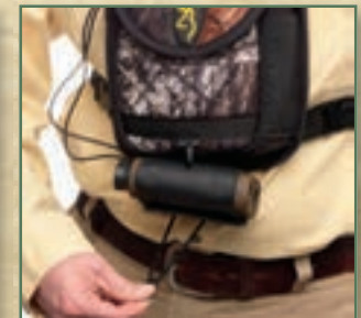
Backup lanyard and security bungee strap secures range finder over rough terrain.
