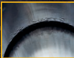
The forcing cone of the competition is pitted and damaged beyond repair after 500 rounds of steel shot.
