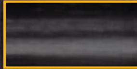
Browning's Invector-Plus choke tube is still flawless after 500 rounds of steel.
