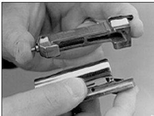
The bolt and bolt slide can be separated for cleaning.
