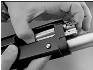
Slide the bolt and bolt slide forward and out of the receiver.
