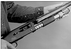
Slide the gas assembly over the magazine tube and the barrel extension into the receiver.
